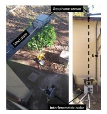
Fig. 4. Experimental setup of controlled environment
