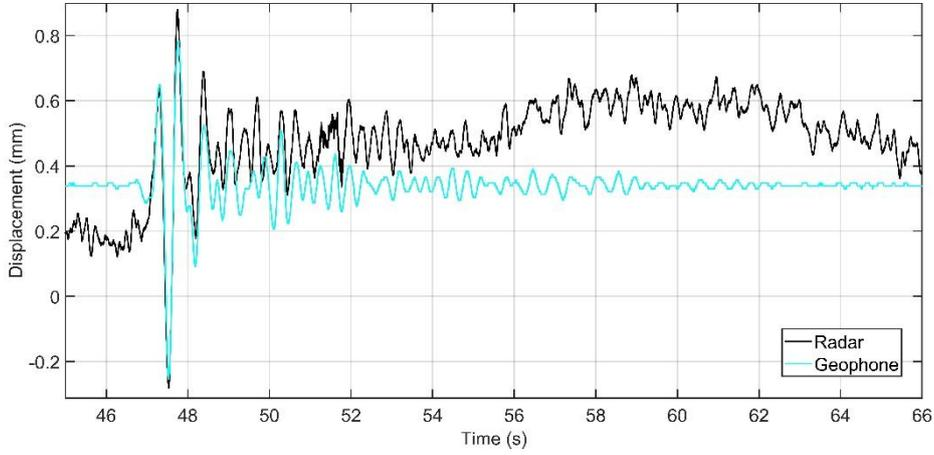
**Fig. 9.** Comparison between displacements measured by the interferometric radar (Black) and the geophone system (Cyan) zoomed on the stimulus by using their own bandwidths.
