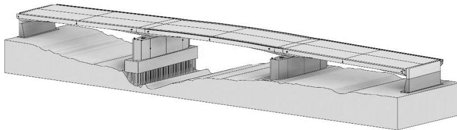
**Fig. 2.** Design of Vespucci bridge with erosion under left pier
