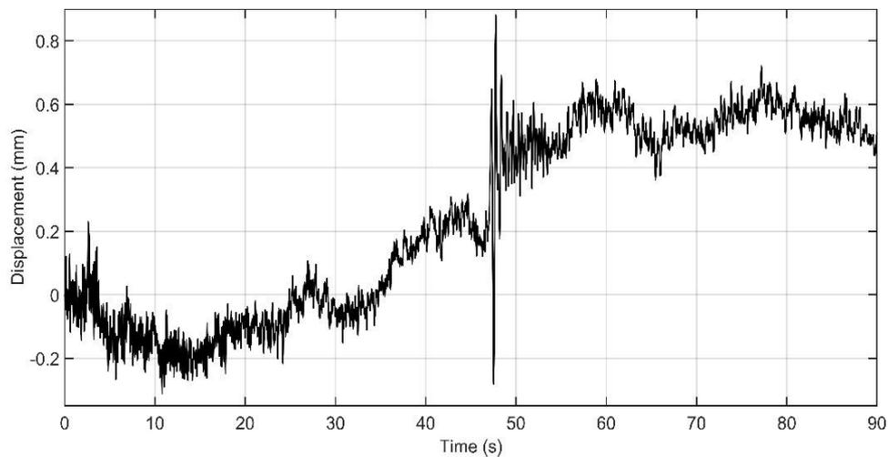
**Fig. 8.** Displacement measured by interferometric radar.
