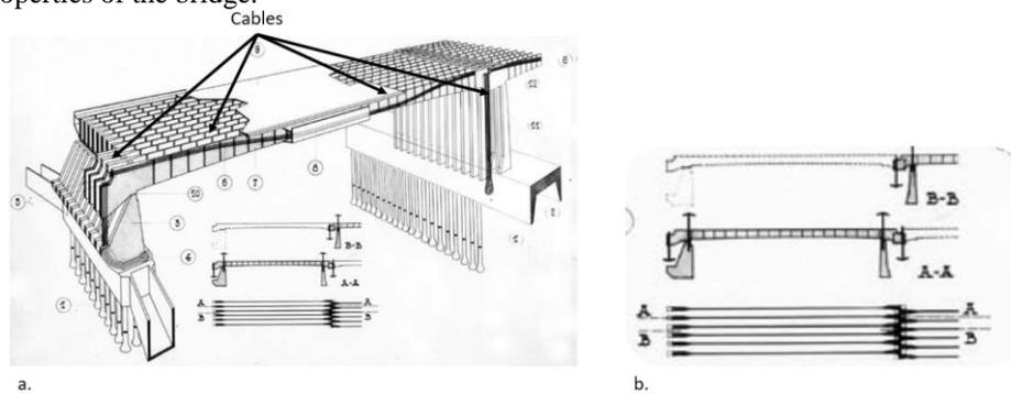
**Fig. 3.** Design of counterweight system of Vespucci bridge (a.). Detail of comb of cables (b.) [11].
