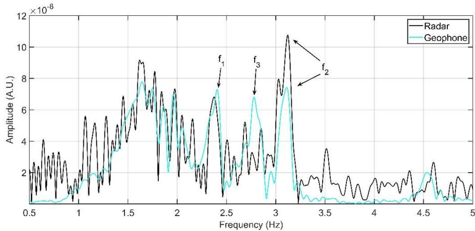
**Fig. 11.** Natural frequencies of Vespucci bridge measured with radar (Black) and geophone (Cyan)
