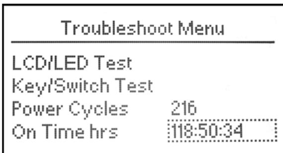
Tests for LCD brightness, contrast, and light or dark pixels. Lights LED's in sequence.
