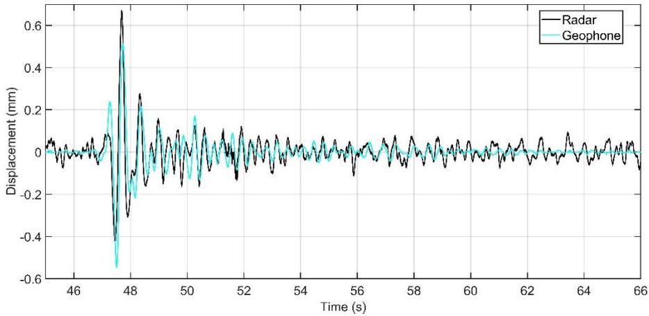
**Fig. 10.** Comparison between displacements in a common bandwidth of interferometric radar (Black) and geophone system (Cyan).
