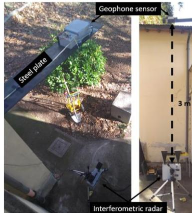
**Fig. 4.** Experimental setup of controlled environment
