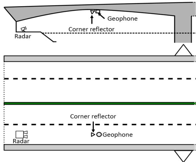
**Fig. 7.** Measurement setup during the dynamic test of Vespucci bridge.
