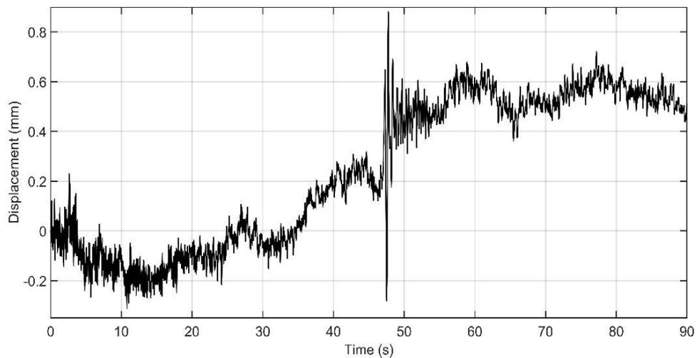
**Fig. 8.** Displacement measured by interferometric radar.
