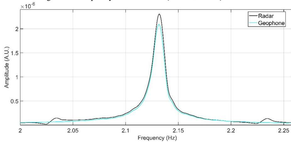
**Fig. 6.** Comparison between frequencies measured with interferometric radar (Black) and geophone system (Cyan).
