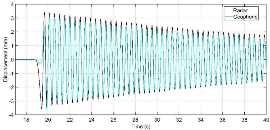
**Fig. 5.** Comparison between displacements measured by interferometric radar (Black) and by geophone system (Cyan).
