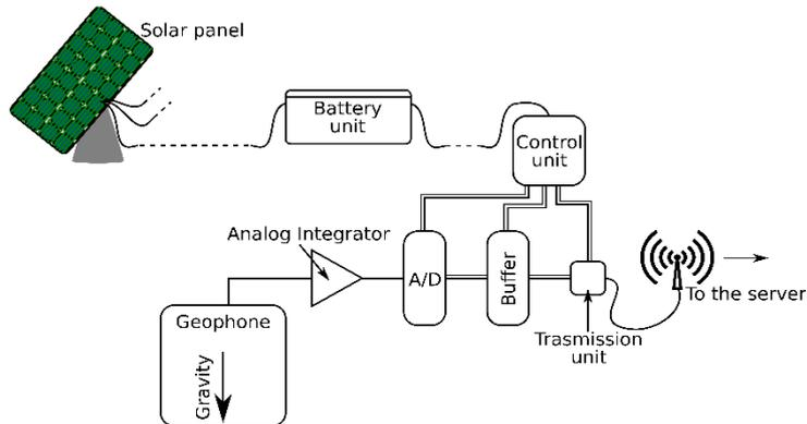
**Fig. 1.** Block scheme of geophone sensor
