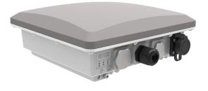
The Gateway Pro is a control unit for receiving and sending data with which, thanks to the LoRaWAN wide-area communication protocol, dozens of devices and sensors can be managed and communicated with simultaneously. This device, first of all, receives the information transmitted by the multiple sensors installed via LoRaWAN. Then, using cellular or LAN connectivity, it forwards this data to online servers.
