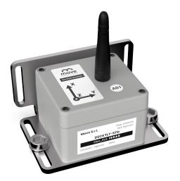
The accelerometer measures the acceleration and temperature of the exact point where it is installed in rela-tion to the structure. It is possible to measure the vibration frequencies and carry out a modal study of the structure. All accelerometers can be perfectly synchronised with each other, perfect for dynamic load tests. Battery power supply and LoRaWAN wireless transmission. The acquisition modes can be set by the user via the web interface provided in the service.
